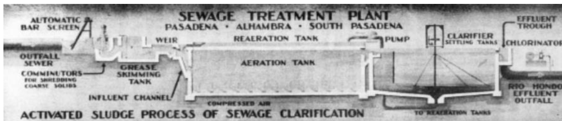
Plan for the activated sludge process at the new Tri-City Sewer Farm. From “Forgotten Facilities: The City of Pasadena Tri-City Sewage Treatment Plant – Part 1.”
